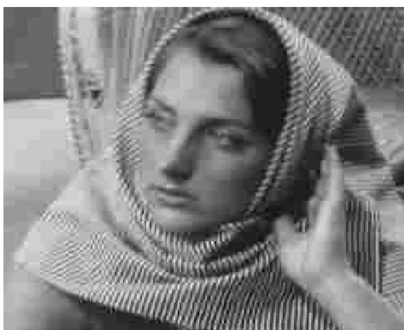
Figure 5.2. DCT Compressed Image
