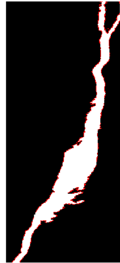
Final Crack of which length and area is calculated
