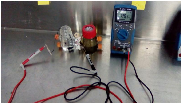
Figure 2 Experimental Setup for a Microbial Fuel Cell
