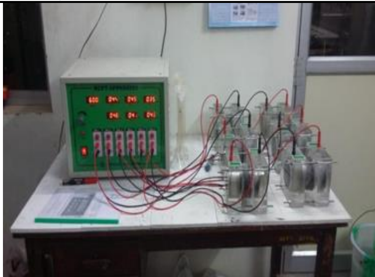
Fig. 8 Rapid Chloride Based Permeability Test Setup
