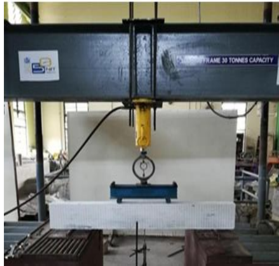
Fig. 5 Test Setup for Two Point Load Test
