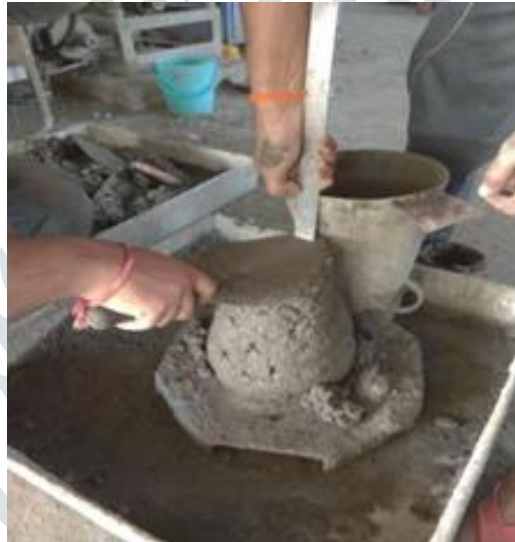
Fig. 4 Testing of Slump
