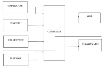
Figure 1: Block diagram of proposed robot for green house monitoring
