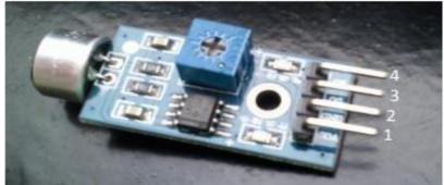
Fig 5: Sound Sensor and its Pin-Out
