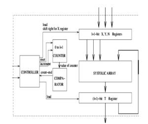
Figure 3: Architecture of the Montgomery modular multiplier circuit
