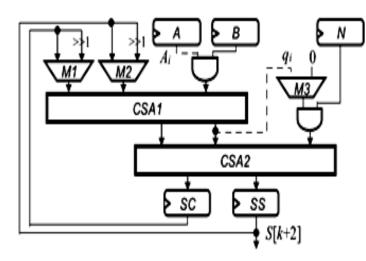
Figure 2: Low cost High performance VLSI architecture
