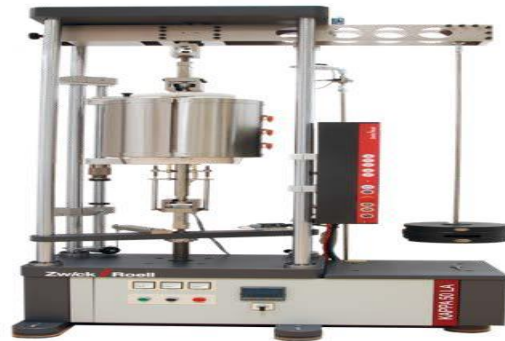
Fig. 2 Existing Creep Tension Machine
