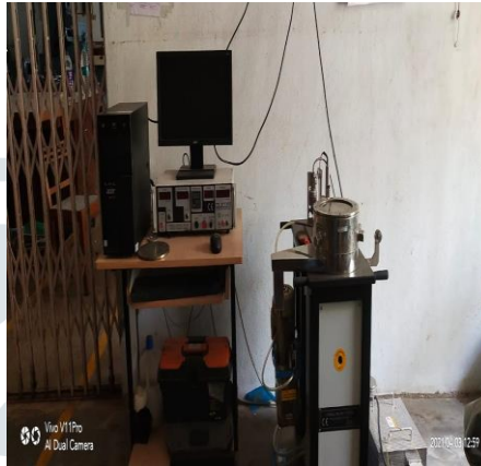
Fig 6 Pin on Disc Sliding Wear Testing machine with an integrated system
