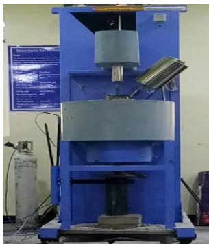
Fig 1 Equipment of Stir casting machine
