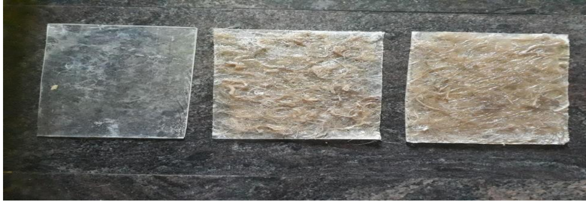
FIGURE 5 FABRICATED COMPOSITES AT 0% FIBERS, 5% FIBERS, 10% FIBERS
