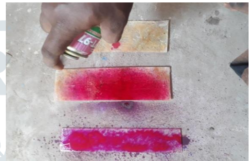
Figure 9 Penetrant (red dye) being applied to the suspected area
