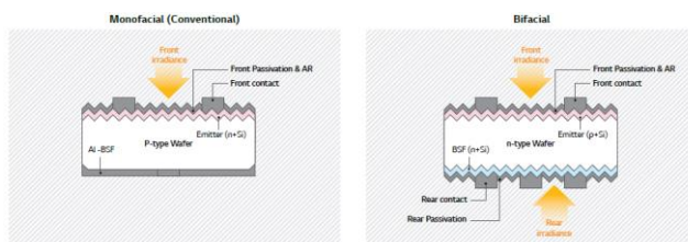
Fig. 3. Difference in Cell architecture between poly-Si (Monofacial) and Bifacial cells ( Ref: LG Electronics)
