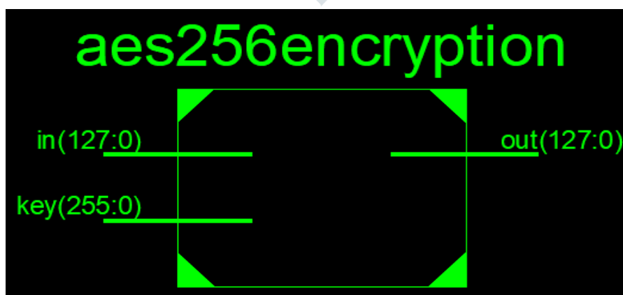
Figure 3: RTL Schematics of WiMax/IOT MAES
