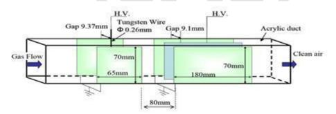
ESPswork by creating a high voltage electrical field (corona) around the discharge electrodes, which causes the gases and the dust particles being carried by the gases, to get ionized. The dust particles, once charged, migrate to and deposit themselves on the neutral collecting plates, from which they are dislodged by periodic rapping and guided to dust hoppers for removal
