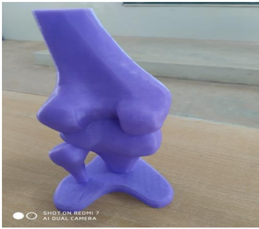
Fig 3 3D printed knee joint bone
