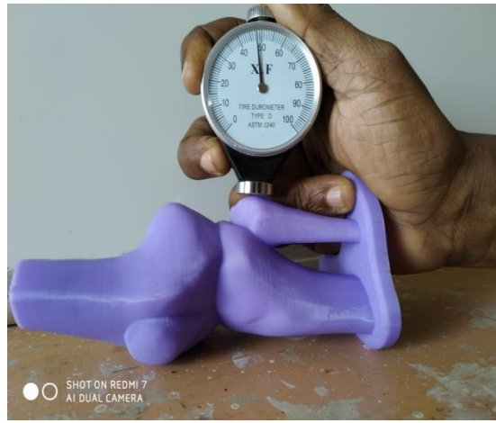
Fig 4 Hardness measurement of SD printed bone
