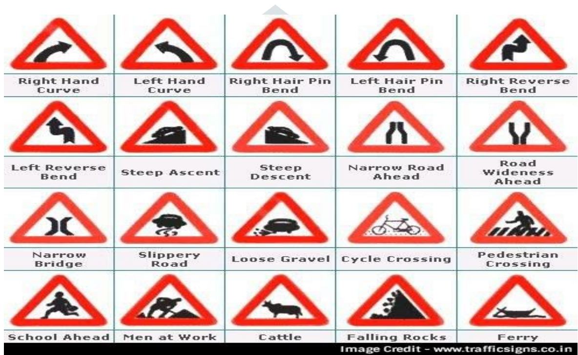
fig.6 Pre warning signs
