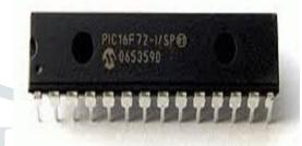
PIC stands for Peripheral Interface Controller given by Microchip Technology to identify its single-chip microcontrollers. These devices have been very successful in 8-bit microcontrollers. The main reason is that Microchip Technology has continuously upgraded the device architecture and added needed peripherals to the microcontroller to suit customers' requirements. The development tools such as assembler and simulator are freely available on the internet at www.microchip.com.
