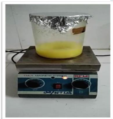
Fig 4 – Buffer Solution on a Magnetic Stirrer
