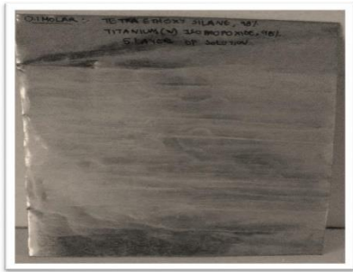
Fig 3 – Five layers coating of solution on Aluminum sheet to check the adhesive property of the base solution
