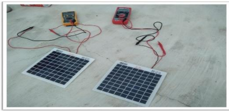
Fig 5 - Comparing Voltage Potentials of Coated and uncoated solar panels
