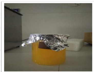
Fig 1- 0.1 molar Titanium Iso Propoxide + Tetra Ethoxy Silane + Pure Alcohol
