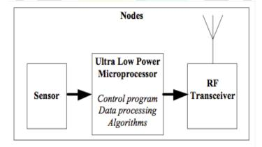
Typically, wireless sensor node consists of sensing, computing, communication, actuations and power components. These components are integrated on a single or multiple boards and packages in few cubic inches. Low power circuit and networking technologies, a sensor node powered by 2AA batteries and last upto three years with 1% low duty cycle working mode.
