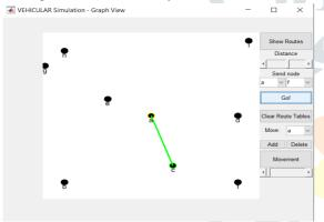
The route which is efficient and fast to send a message to receiver can be discovered by selecting the sender and receiver nodes and clicking the Go button. The Show Routes button gives all possible routes from the sender to receiver node.
