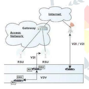
RSU (Road-Side Unit) DSRC communication unit that is located aside the roads. It serves as a gateway between OBUs and the communications infrastructure.
