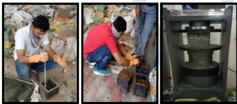
Fig. 1.3 Cube Compressive Strength Test
