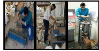
Fig. 1.4 Beam Flexural Strength Test
