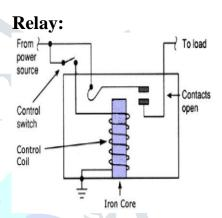
Relays are simple switches which are operated both electrically and mechanically. Relays consist of an electromagnet and also a set of contacts. The switching mechanism is carried out with the help of the electromagnet. There are also other operating principles for its working. But they differ according to their applications.
