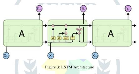
In the above diagram, each line carries an entire vector, from the output of one node to the inputs of others. The pink circles represent pointwise operations, like vector addition, while the yellow boxes are learned neural network layers. Lines merging denote concatenation, while a line forking denotes its content being copied and the copies going to different locations [15].
