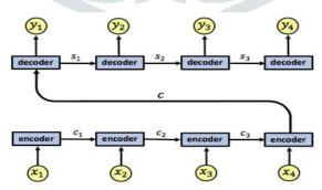
Figure 1: Encode-Decoder Architecture
