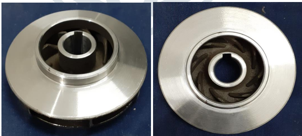
Figure 3.0.1 : Impeller manufacturing via sand casting method
