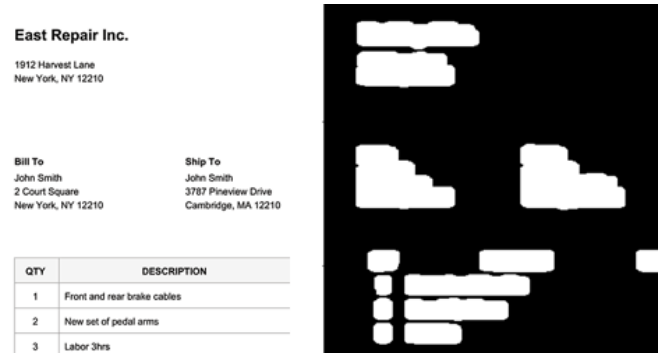
Figure 2: The binary grayscale output obtained after preprocessing the raw image
