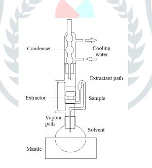
Figure 2: Soxhlet apparatus
