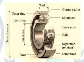
Camshaft Bearing Bigger End code: 6203
