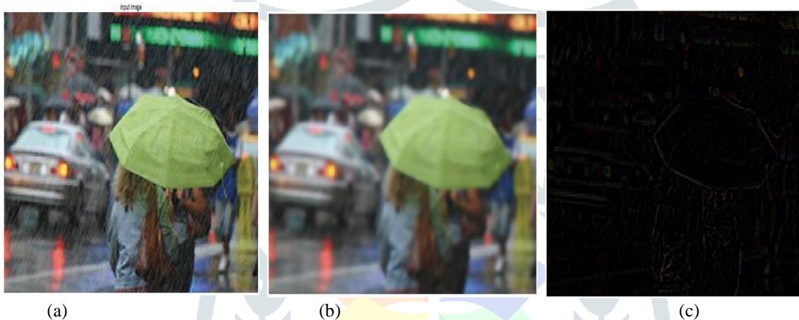
Fig 5. (a) Input Image (b) Low Frequency Components of Rain Image (c) High Frequency Components of Rain Image Now the three level classification results are obtained and shown in Fig 6.
