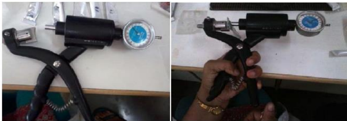
Figure 5: Extrudability Studies Using Pfizer Hardness Tester
