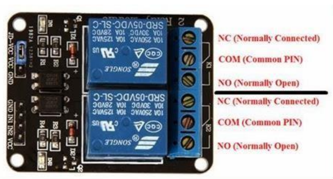
Figure no. III.3 Relay
