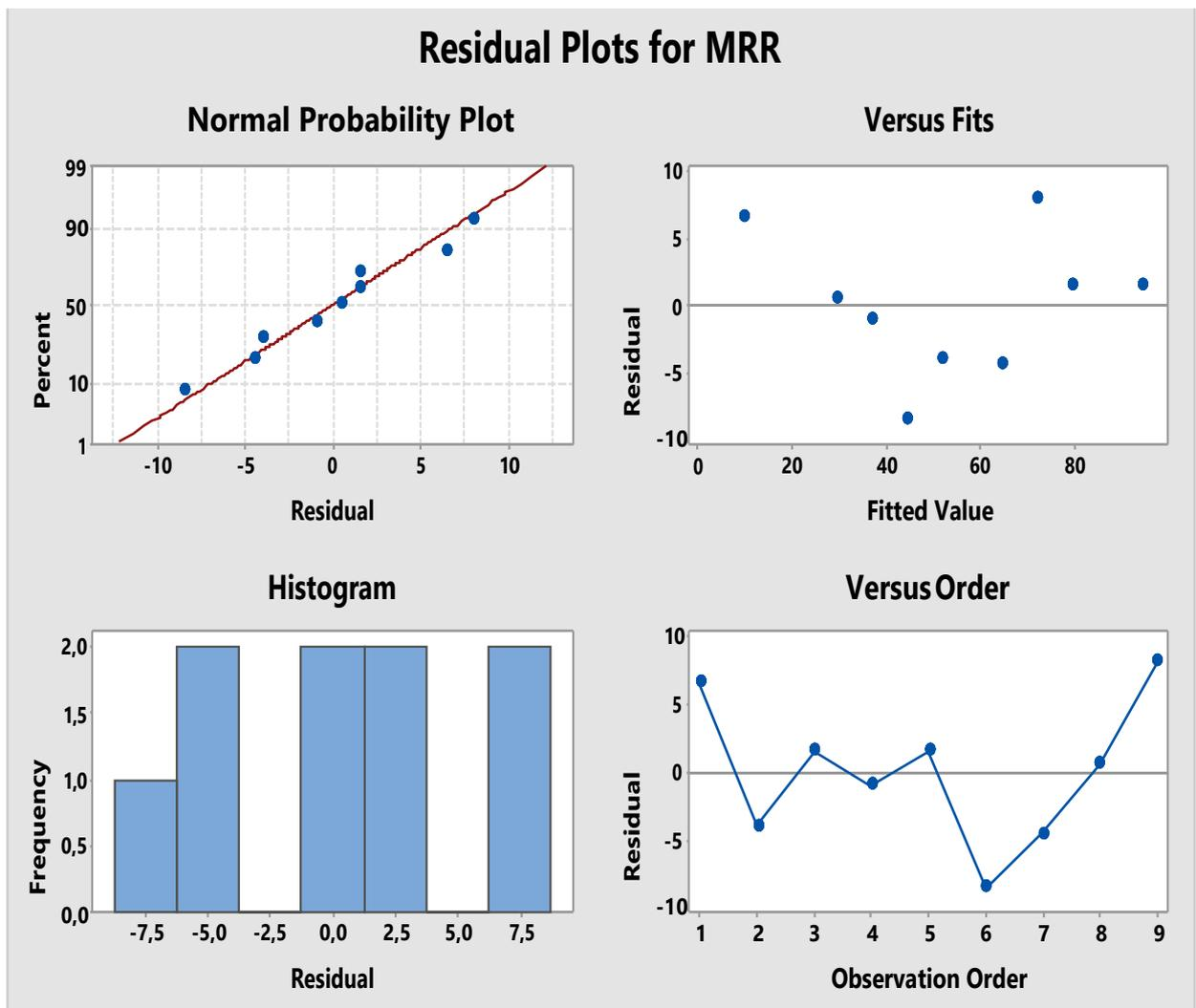
Fig. 4.2. Residual plots for material removal rate.
