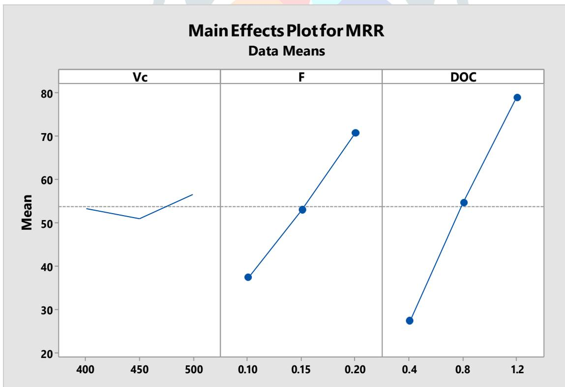
Fig. 4.4. Main effects plot for material removal rate.
