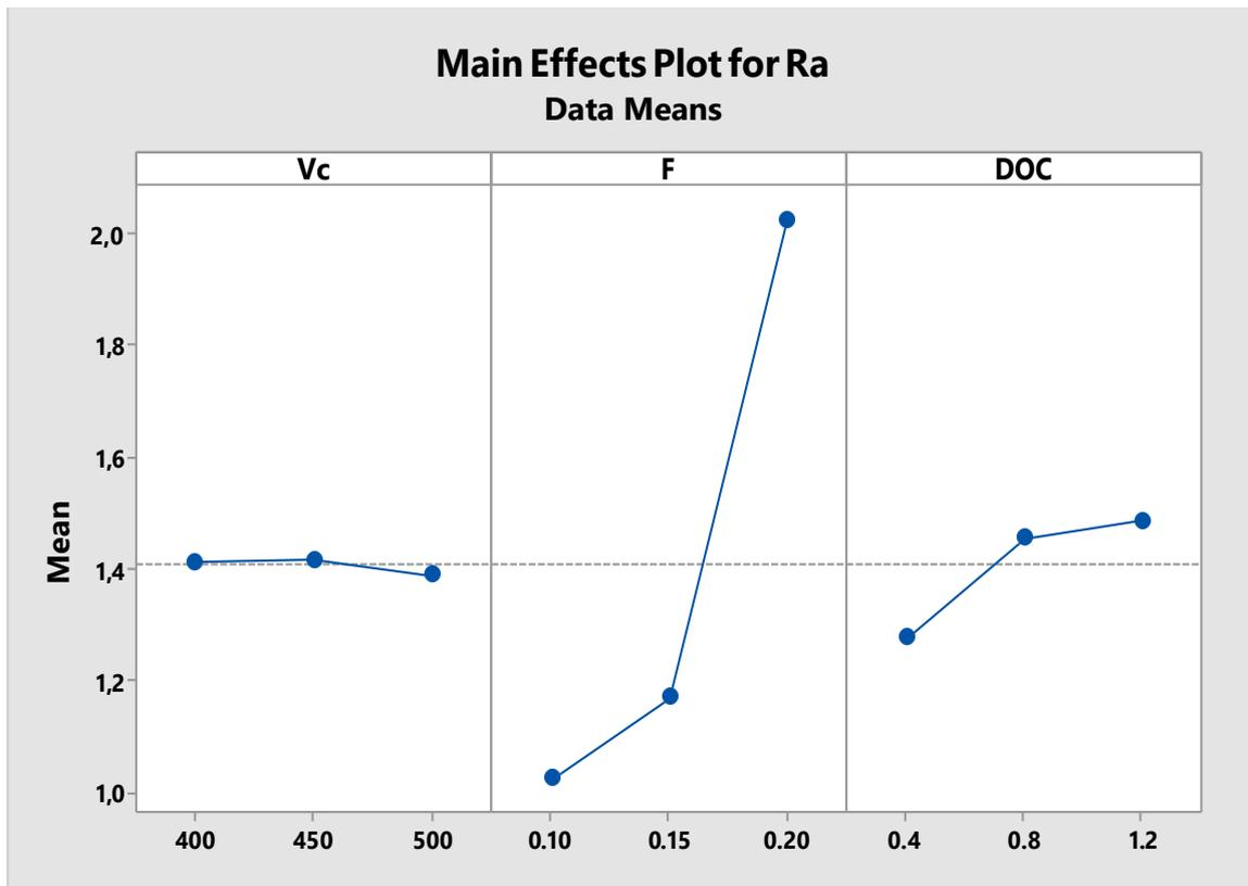
Fig. 4.3. Main effects plot for surface roughness.
