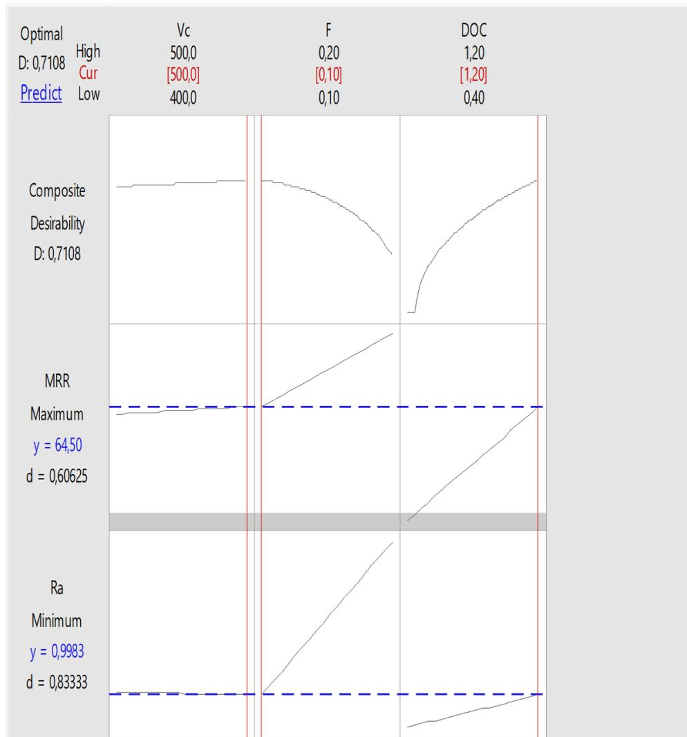
Fig. 4.5. Optimized plots for surface roughness and material removal rate.
