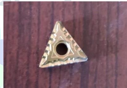
Fig. 3.2. Cementite Carbide Tool Insert (CJ225P)
