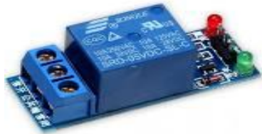
Fig: 5V 10A 1 Channel Relay Module for Arduino
