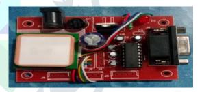
The GPS Receiver consists of two units, first is active antenna which receives RF signals and amplifies it. The antenna is active in the sense it takes power from the module and amplifies the signal for high sensitivity. The RF signal is filtered and processed to generate NMEA format serial data output.
