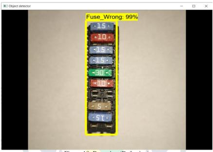
Figure 18: Detection (Defective)
