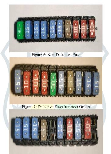
Figure 8: Defective Fuse(Missing fuse)
