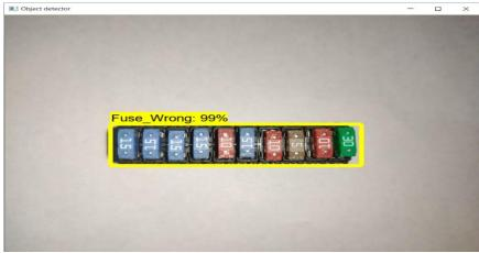
Figure 17: Detection (Defective)
