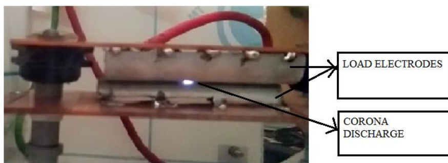
Fig.3 Corona Discharge shown between plates kept at 1mm distances
