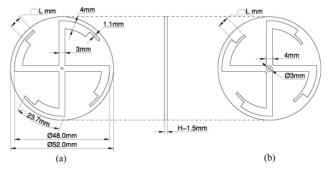
Figure 1. Geometrical structure presentation of the proposed antenna (a) top view (b) bottom view
