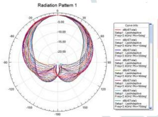
Figure 3: Radiation Pattern of F-shaped
