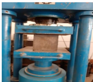
Figure II: Specimen under a CTM
