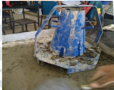
Figure V: Slump Cone with Base plate attached to it.
