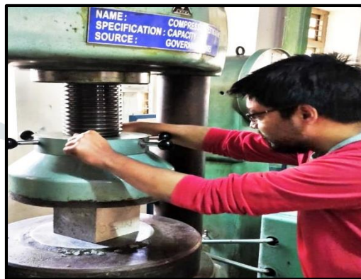
Figure 7 Compressive strength test
