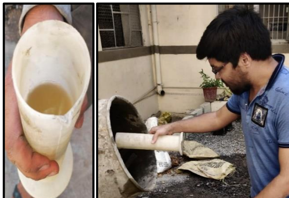
Figure 6 Addition of bacterial liquid during concrete mixing by direct application method
