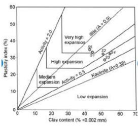
This chart classifies the soil into active, normal and inactive soils on basis of plasticity index and clay fraction present in soil. It is desirable to first check sample on this chart to see that the soil does not full into active zone. As per the suitability the soil sample identified on this chart i.e. not falling into active zone shall be checked on plasticity chart with below procedure.
