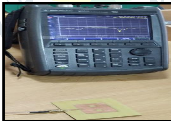
Fig. 9. Measurement of hardware result using Network Analyzer
