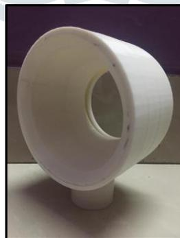
Fig.10. 3D printed Prototype 2 Thruster with three components.
