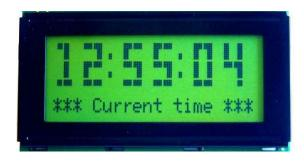
One of the most common devices attached to a micro controller is an 16x2 LCD display. This means 16 characters per line by 2 lines and 20 characters per line by 2 lines, respectively. The project status will display on LCD.
