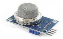
Air quality **sensor** for detecting a wide range of gases, including NH3, NOx, alcohol, benzene, smoke and CO2. Ideal for use in office or factory. MQ135 gas sensor has high sensitivity to Ammonia, Sulfide and Benze steam, also sensitive smoke and other harmful gases. to The **MQ135** Air Quality **Sensor** consists of a small **sensing** material whose conductivity is lower in clean air and higher in polluted air, thus
