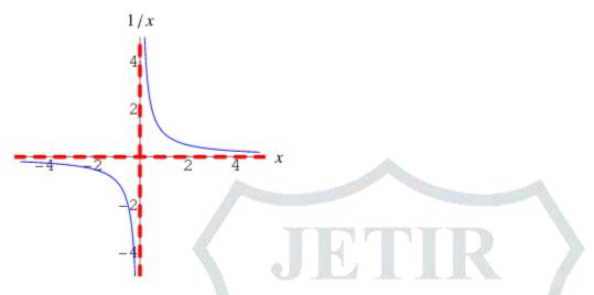
The plot above shows 1/x, which has a vertical asymptote at x = 0 and a horizontal asymptote at y = 0.
