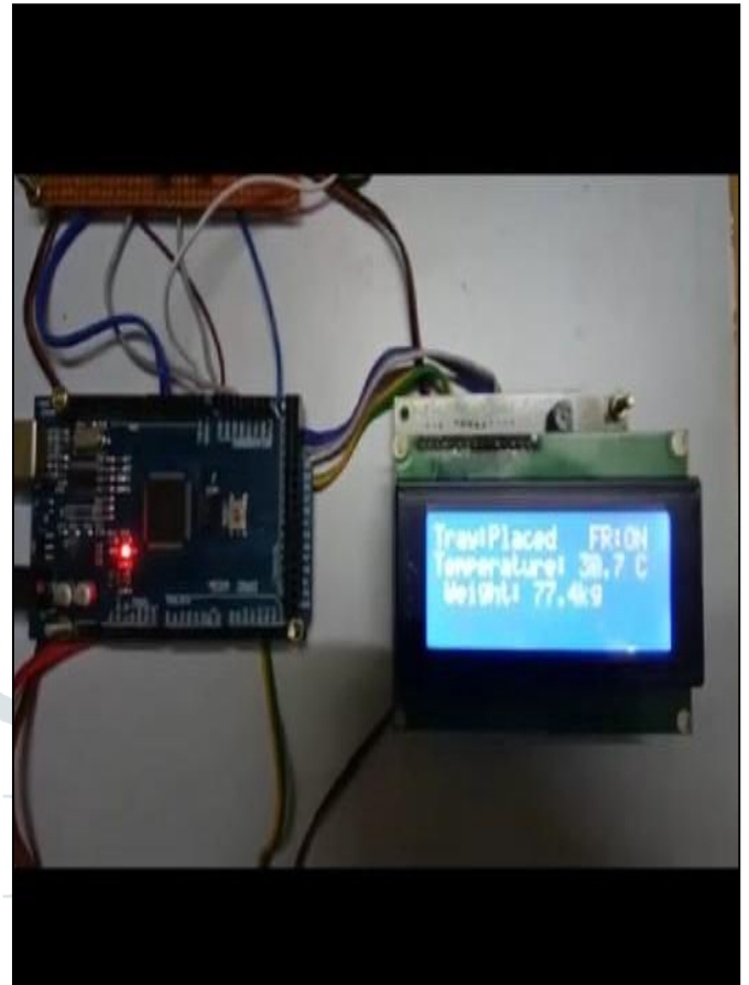
figure 6 : status displayed on lcd
