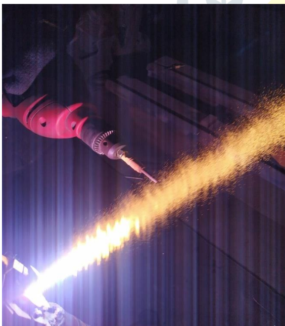
Fig.2 PSZ Plasma coating on glow plug heating rod
