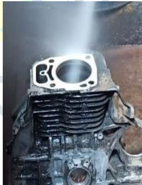
Fig.8 Grinded Engine Bore
