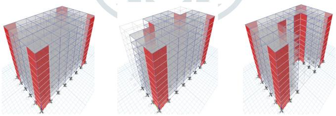
Fig 1. Elevation view of 10 storey having shear wall (a) Rectangle (b) T-shaped (c) C-shaped
