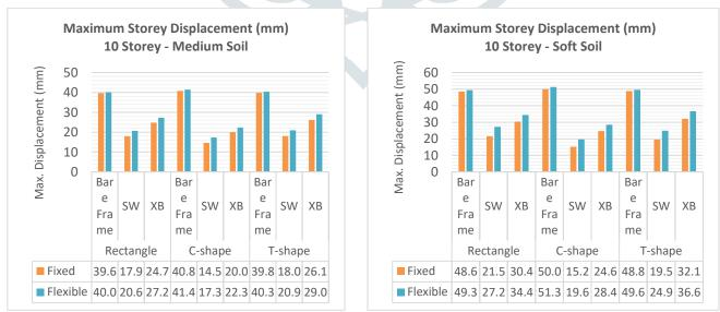
Maximum Storey Displacement (mm) of 10 Storey: (a) Medium Soil (b) Soft Soil
