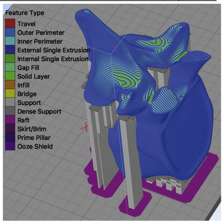
This is a digital image created by "Simplify3D" software. The varying colors demonstrate different print processes. The support material (light gray, dark gray) and raft (purple) facilitate the printing process and are removed from the model after print completion. Image created is taken by the reference papers
