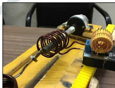
Figure 7 Feasibility with Circular Coil in Rotating workpiece
