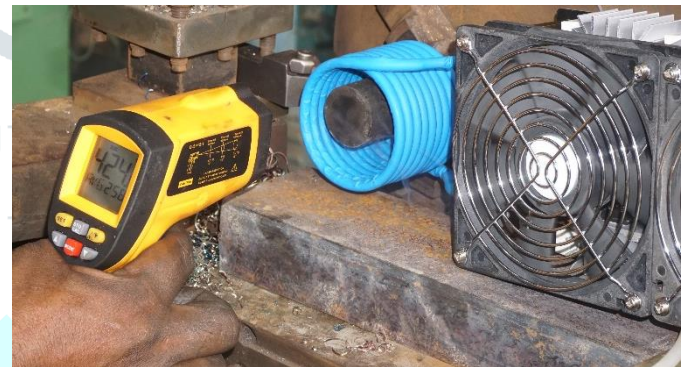
Figure 20 Temperature Sensing During Pre Heat
