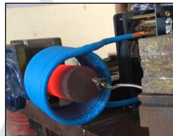
Figure 14 Heating check at 600°C
