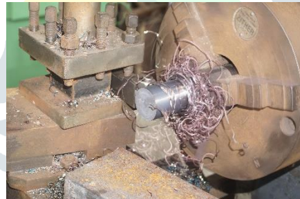
Figure 23 Smooth Chip Formation during machining
