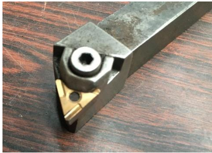
Figure 3 Ceramic Cutting Tool with TNMG8135 grade
