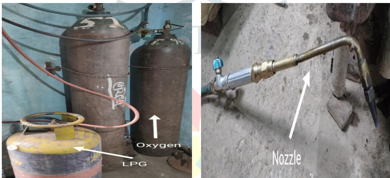
Figure 1: Experimental setup of flame brazing (Heat source and nozzle )
