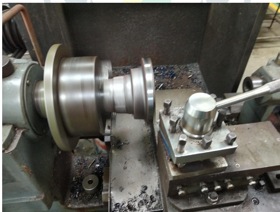
Figure 5: Face clean cut operation and process parameters
