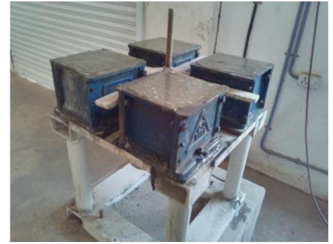
Fig.3 Compaction of concrete
